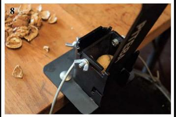
**8.** To fix the Nutcracker - Nut Crusher Steel, on the table or the workbench, just screw it, through the two holes in its base. Now you are ready to use it!
