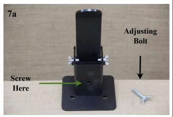
7. Place the Adjusting Bolt at the back of the Main Body and screw it according to the size of the nuts you will break. The Adjusting Bolt tightens the walnuts or other nuts until they lock between the Metallic Lever and the Metallic Face Plate. (Photos 7a, 7b, 7c, 7d & 7e)
