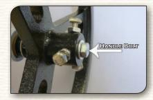
**11.**Put the handle bolt and washer back onto the shaft and tighten bolt.
