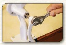
**1.** Remove milling heads and handle bolt.
