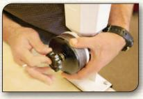
**3.** Install stainless steel milling heads (DO NOT USE the STONE MILLING HEADS - they might crack).
