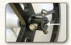
9. Make sure the 3 set bolts are lined up with the 3 flat spots on the shaft and that the shaft end is flush with the Pulley Attachment (IT MUST NOT PROTRUDE BEYOND PULLEY SURFACE).
