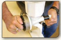
**4.** Tighten adjustment knob until milling head just touch.
