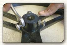
**6.** Loosen all 3 lock nuts on all 3 set bolts on Pulley Attachment.
