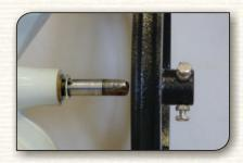
**8.** Slide the Pulley Attachment onto the shaft with the set bolts facing away from the mill body.
