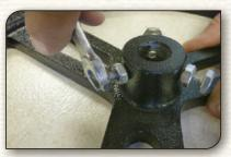
7. Loosen all 3 set bolts until they no longer protrude into center hole.
