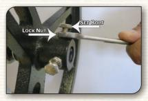
**10.**Tighten all 3 set bolts snug (do not over-tighten). Tighten all 3 lock nuts on all 3 set bolts.
