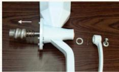
3 Slide auger shaft from mill body.
