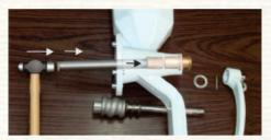
**4** Using a long flat punch, gently tap old bearings from mill body by tapping from the inside of the mill so old bearings will fall out from the handle side of the body.
