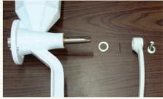
**2** Remove pin from auger shaft and remove race washer.
