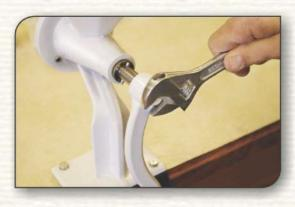
1. Remove milling heads and handle bolt.
