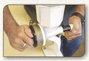
4. Tighten adjustment knob until milling heads just touch.
