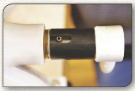
2. Place handle remover on shaft with handle pin through slot.
