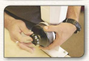
3. Install stainless steel milling heads. DO NOT USE the STONE MILL-ING HEADS, as they may crack.
